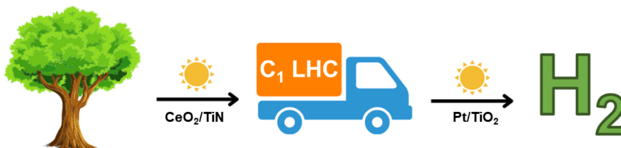
Figure 1. Illustration of H 2 production from biomass and storage in the form of LHCs by a stepwise method.
